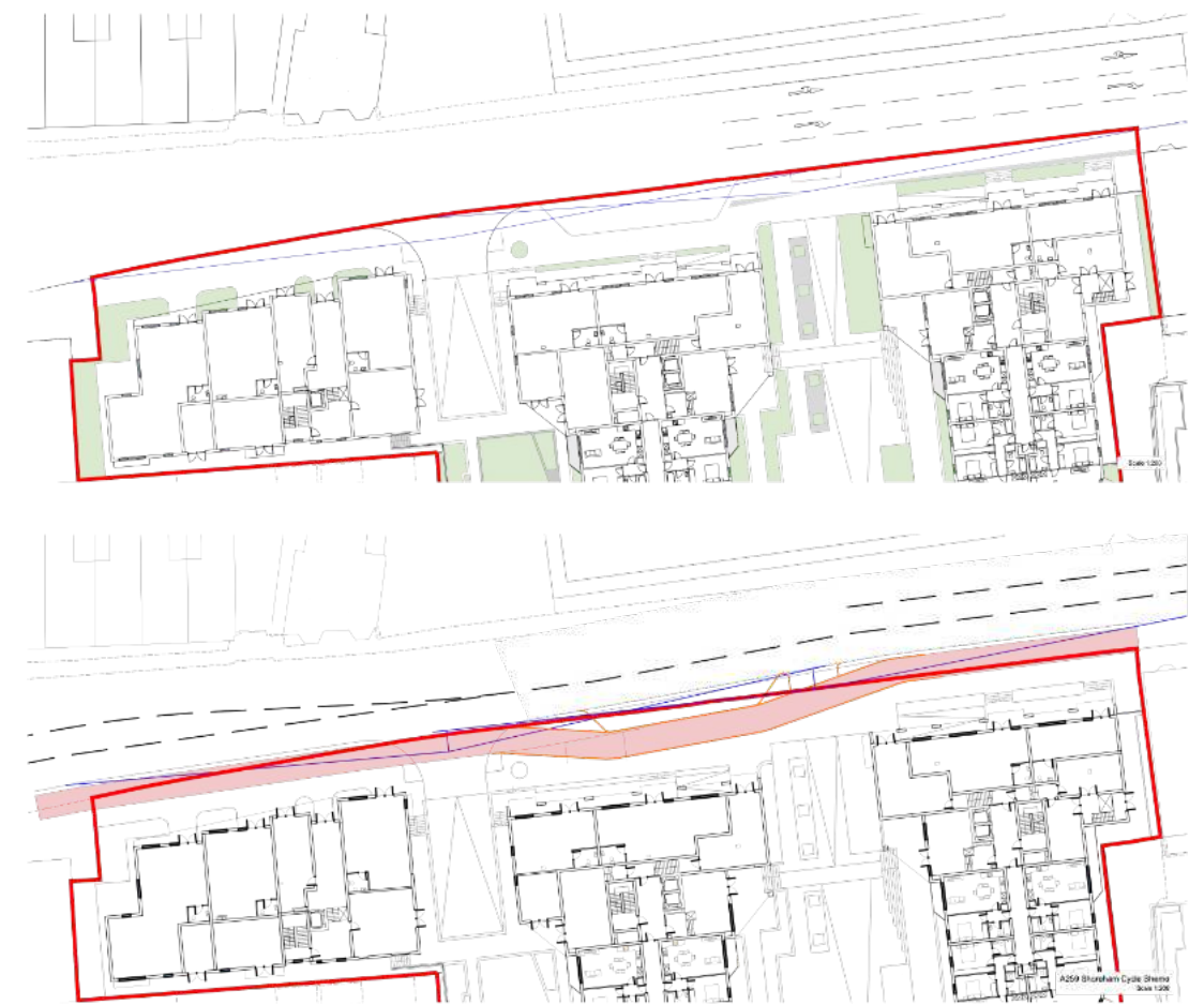
The site's road frontage, both as it will be constructed initially (top image) and as it will be in the future, when the new cycle lane is constructed on Brighton Road.
